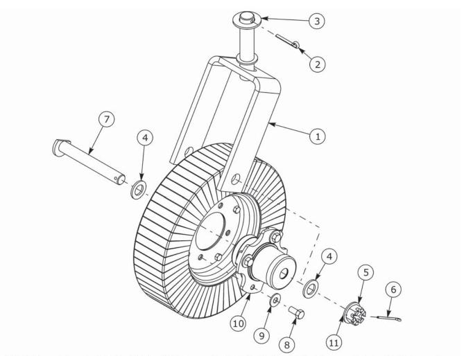
NOTE: Items 5-9 are included in Tailwheel Hub Assembly (00780238). For detailed view see Tailwheel Hub Assembly Page.
