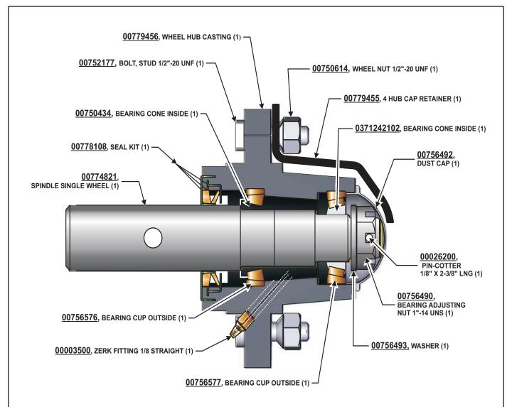
NOTE: If your unit uses this hub the hub will be equipped with zerk fitting 00003500.
