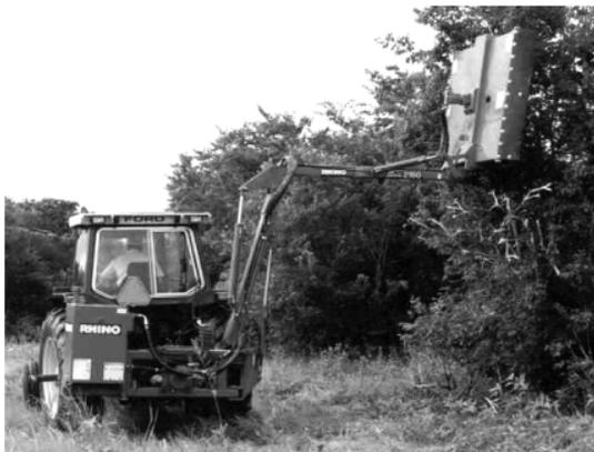
The Servis 2160 is designed for agricultural applications including cutting grass, weeds, and material up to 2" in diameter on an intermittent basis.
