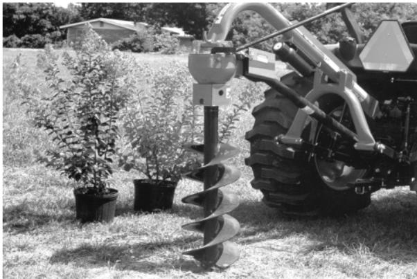
Rhino offers 4 models of pto driven post hole diggers for CAT I & II hitch tractors.
