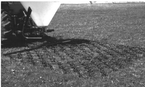
Fuerst F-L-E-X-I-B-L-E Tine Harrows® are built tough and require virtually no maintenance. Applications include pasture renovation, herbicide and fertilizer incorporation, seedbed preparation; and racetrack, ball diamond, arena, and park trail maintenance.
