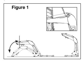
Using overhead hoist to support loader, disconnect and remove angle support strut and install 2 inch lift cylinders (8). Fasten hydraulic hoses to cylinder ports.
