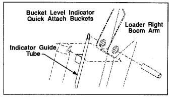
Slide bucket level indicator rod through guide tube. Attach other end of rod with 1/8 x 1 cotter pins. If pin on bucket is used, attach lower end of rod to bucket ear. If quick attach device is used, attach lower end of rod to quick attach device.
