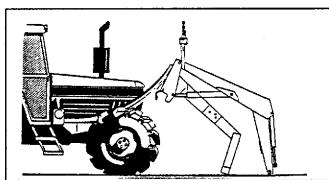
6. Start tractor engine, release tractor brakes and slowly drive forward while operating lift control levers to retract lift cylinders. Position loader so hinges hook over mid mounting tubes. Use of overhead hoist will facilitate positioning loader into mid mounting tubes.
