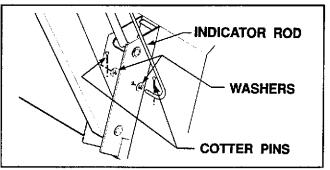
Locate tractor and loader on level surface. With bottom of bucket resting on surface, cut off excess rod flush with end of guide tube or paint exposed rod a contrasting color.
