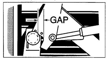
**IMPORTANT:** Position loader uprights so mid mounting tubes are tight against hinges until loader has finished rotating so loader front bumper tube does not hit lower flange of front mounting channel.
