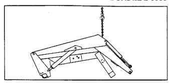
5. Operate loader control valve to extend lift cylinders until front yoke is resting on ground and side frame uprights will clear front tires. Shut off tractor engine and engage tractor brakes. Reroute loader hoses to inside of right midmount bracket. Remove locknut and washer from loader hinge and swing each hinge open.
