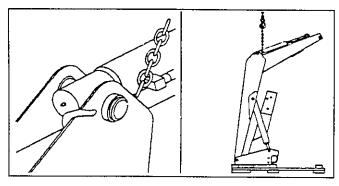
Using overhead hoist, lower loader from vertical shipping position to horizontal position leaving enough room to install yoke (scraps of cardboard may be used to protect paint). Install yoke assembly (5) using 3/4 x 2-1/2 cap screws (12) and 3/4 lock nuts (10). Lower loader completely to the ground.
