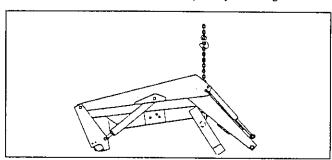
**NOTE:** Hardware connecting yoke to loader sideframes should be snug but do not torque completely. After loader has been mounted to tractor and aligned with midmounting brackets and front mounting brackets, torque hardware to specifications in loader operators manual.
