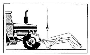
Start tractor engine, release tractor brakes and slowly drive forward while operating lift control levers to retract lift cylinders. Position loader so hinges hook over mid mounting tubes. Use of overhead hoist will facilitate positioning loader into mid mounting tubes.
