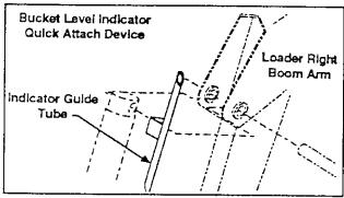
2. Slide bucket level indicator rod through guide tube. Attach other end of rod with 1/8 x 1 cotter pins. If pin on bucket is used, attach lower end of rod to bucket ear. If quick attach device is used, attach lower end of rod to quick attach device.
