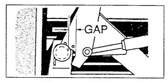
**IMPORTANT:** Position loader uprights so mid mounting tubes are tight against hinges until loader has finished rotating so loader front bumper tube does not hit lower flange of front mounting channel.
