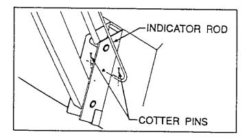
Locate tractor and loader on level surface. With bottom of bucket resting on surface, cut off excess rod flush with end of guide tube or paint exposed rod a contrasting color.
