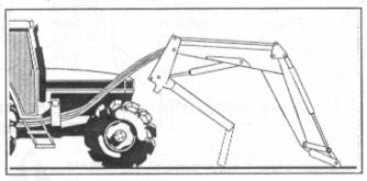
WARNING: When loader is mounted on a tractor with super steer, use caution when maneuvering in tight quarters at very slow ground speed or when tractor is stationary. Tractor frame will shift in the opposite direction from the steering direction. Front of loader bucket may move as much as 10-12 inches opposite of steering direction before it starts to move in the direction the wheels are turned.
