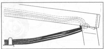
Wrap one rubber strap twice around hoses and oil line between cab and front of rear tire.
