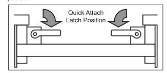
6. Start skid steer engine and activate lift cylinders to raise pallet fork two or three feet off ground and extend tilt cylinders at a slight downward angle, so quick attach latch pins are visible. Visually inspect attachment mechanism to verify that pins are engaged through latch plate at bottom of pallet fork attachment pads.
