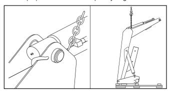
**NOTE:** Hardware connecting yoke to loader sideframes should be snug but do not torque completely. After loader has been mounted to tractor and aligned with mid mounting brackets and front mounting brackets, torque hardware to 239-262 ft. lbs.
