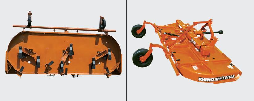
The optional shredding kit on the TW168 features 12 free swinging and 4 stationary blades for increased shredding action. The "baffling" included in the kit helps deflect material into the cutting chamber and evenly distribute the shredded material across the width of the machine.
