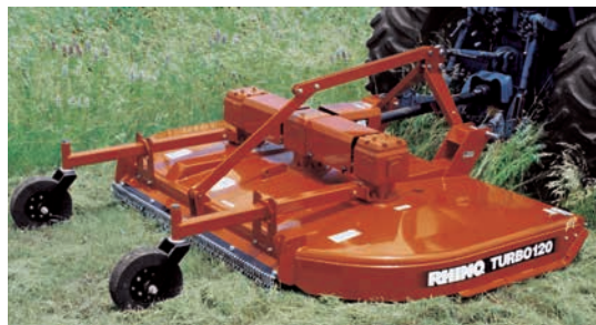
Lift-type units are perfect for working in tight spots where the maneuverability of a mounted cutter is required. (unit shown with optional equipment)
