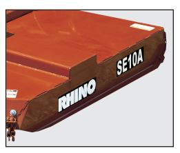
**SIDE SKIRTS AND SKID SHOES:** Replaceable skid shoes are standard equipment to help reduce wear on the side skirts. All gearboxes and drivelines are fully shielded for greater safety. Front and rear rubber safety deflectors are standard. Chain guards are optional equipment.
