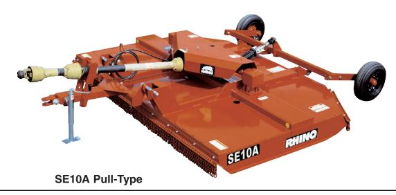
The pull-type SE10A requires only a 45 HP (min.) tractor for economical, wide-cut mowing. A hydraulic cylinder or ratchet lift screw is available for raising and lowering the mower. A spring shock absorber is optional to help cushion shockloads to the mainframe when operating in rough terrain. (Unit shown with optional chain guards. Deflectors are standard.)
