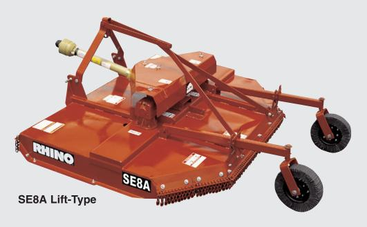
The lift-type SE8A features a CAT II hitch and is designed for use on 540 RPM tractors as small as 45 HP (with adequate front weights). Designed to mow a 94" swath, updraft blades and a 4" blade overlap help ensure a clean cut. The 10 gauge deck and 8-1/2" side skirts are reinforced to help provide dependable mainframe strength.
