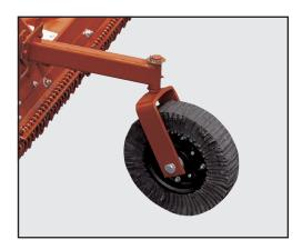
**TAILWHEEL ASSEMBLY:** Lift-type units feature laminated tailwheels for dependable service. Greaseable tapered roller wheel bearings and caster forks are standard for long service life. The tailwheels can be easily adjusted to different mowing heights to help provide the desired cut in your specific application.
