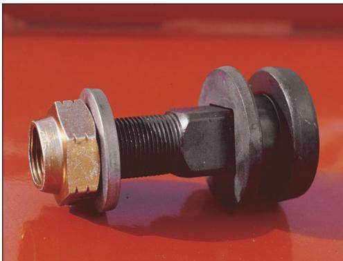
Square shouldered blade bolts are standard on the Rhino TW120 and TW144 for long lasting durability. The square shoulder means that the bolt cannot turn in the blade carrier providing less risk of premature wear compared to round shoulder blade bolts used on most competitive cutters. Round shouldered blade bolts have a small "pressed" key formed on the side. If the key wears or shears off there is little to prevent the bolt from turning in the hole, which can ruin the blade carrier.
