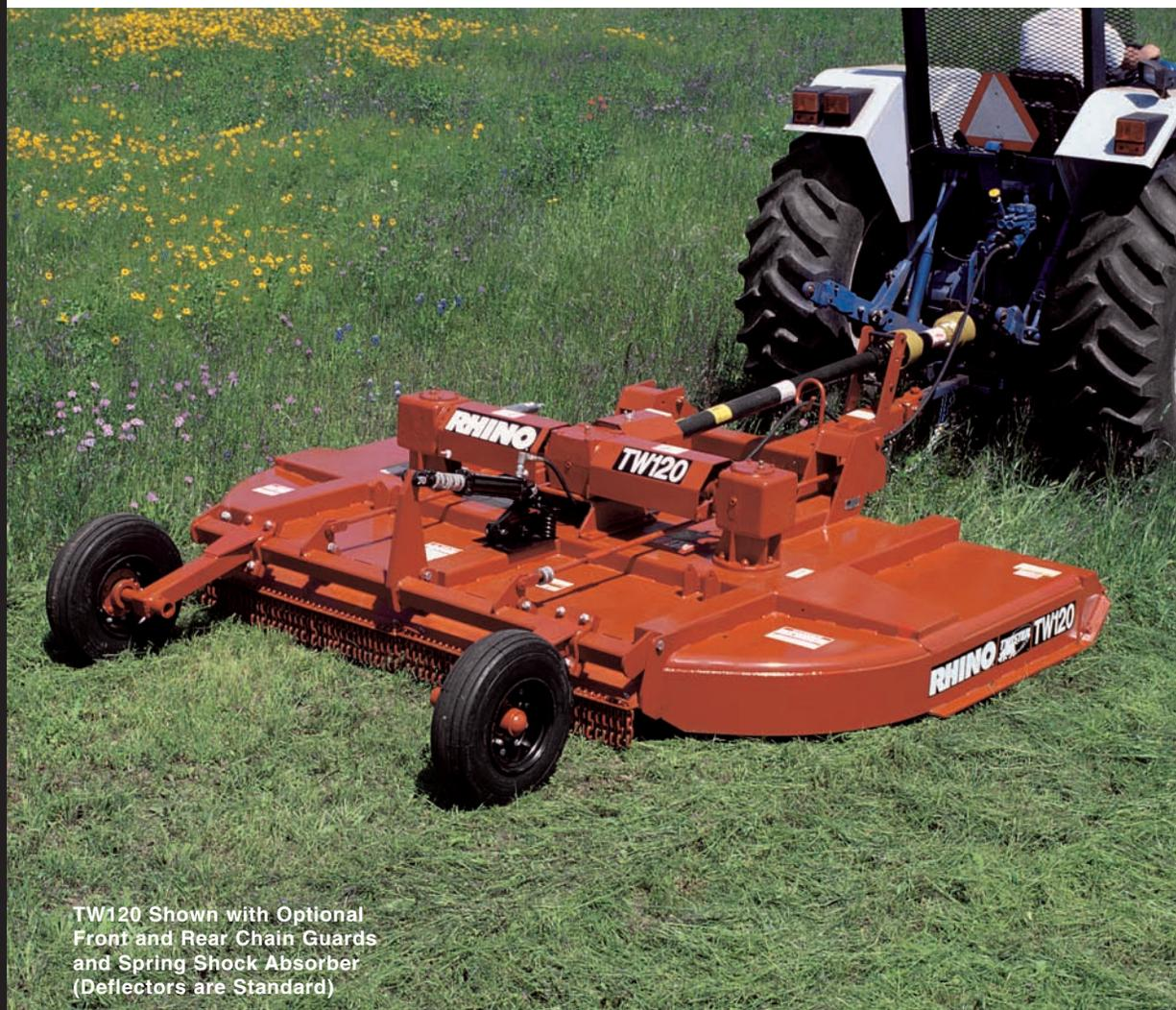
TW120 Shown with Optional Front and Rear Chain Guards and Spring Shock Absorber (Deflectors are Standard)
