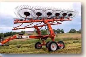
Narrow transport width of only 9'-2". Hydraulics adjust the rake arms from working position to transport.
